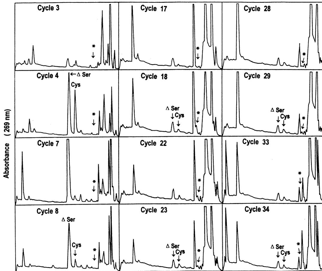
Fig. 4. HPLC profiles of sequencing samples before and after modification with 4-VP after cycle 4 and cycle 8. Conditions as in Fig. 3. Small Pth-PECys peaks are seen in cycle 18 and 29.
